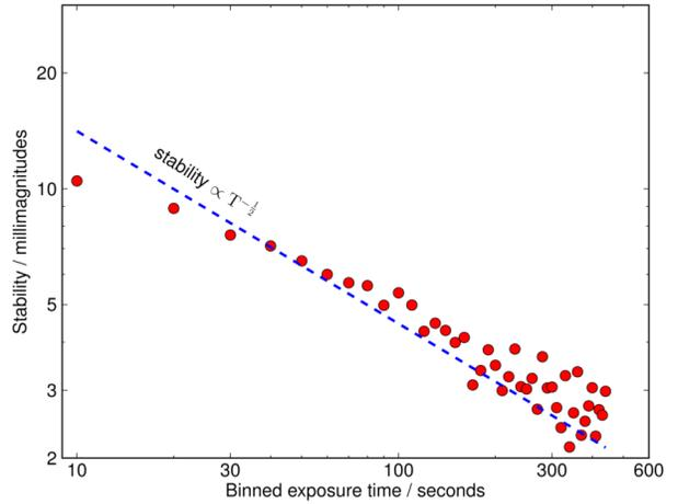
FIG. 2.— *Left*: The AWCam Arctic wide-field exoplanet search telescopes and the first sunrise after a full winter of unattended operation. *Right*: Photometric precision as a function of binning timescale for one of the AWCam telescopes, showing exoplanet-detection levels of photometric stability over periods of months.
