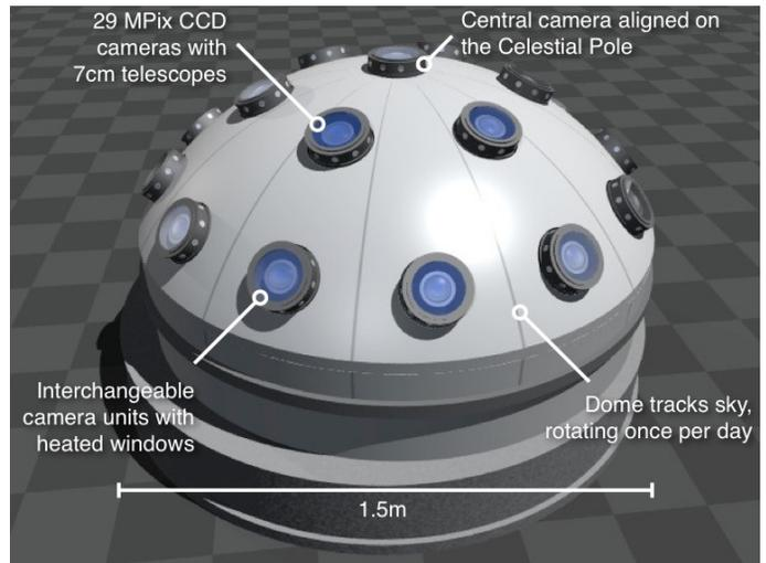
FIG. 1.— The Antarctic Evryscope concept. This example 1.5m-wide dome contains 20 separate 7cm telescopes, delivering a 10,000-square-degree instantaneous field of view with continuous tracking throughout the winter. The concept easily scales to larger apertures and improved sky sampling.
